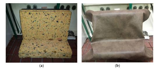
Figure 2. Test equipment. (a) underlying panel and (b) upholstery for the experiment.
